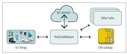
FIGURE 1. A hub architecture for Internet-based IoT (e.g., as adopted in Hypercat [4]).
