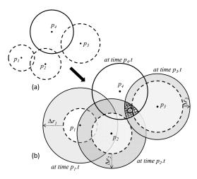
Fig. 3: Example on TSM technique. (a) The set of detections  $P = \{p1, p2, p3, p4\}$  for a tag t at different times within the same tolerance interval where p4 is the most recent. (b) The set of shifted detections after expanding p1, p2, p3 by  $\Delta r1$ ,  $\Delta r2$  and  $\Delta r3$  respectlively, the tag t is expected to be in the shaded area.
