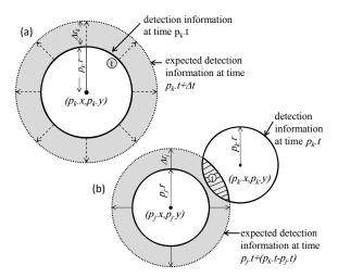
Fig. 4: The concept of time-shifting process. (a) time-shifting of one detection after time  $\Delta t$ . (b) How time-shifting affects location accuracy
