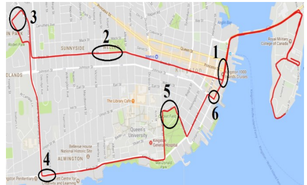
Figure 5. Road experiment in Kingston, ON, Canada, with 6 GNSS Outages.
