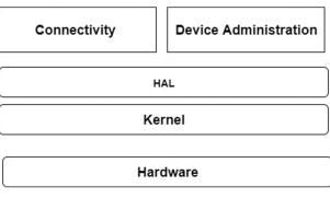
Fig. 11 Architecture of Android Things OS (reproduced from [111])
