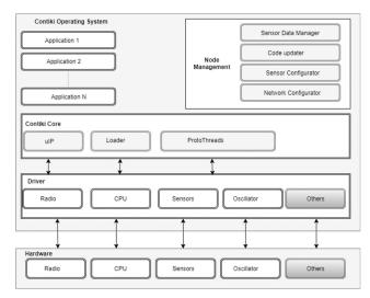
Fig. 4 Architecture of Contiki OS (reproduced from [27])
