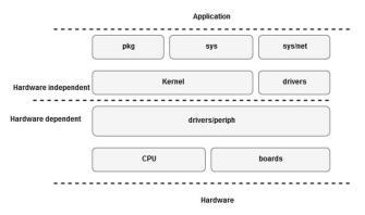
Fig. 5 Architecture of RIOT OS (reproduced from [66])
