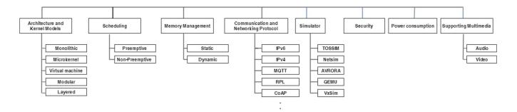
Fig. 1 Overview of the designing and developmental aspects of IoT OSs
