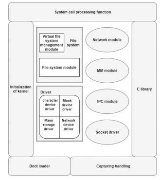
Fig. 9 Architecture of uClinux OS (reproduced from [96])
