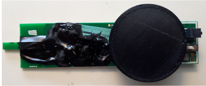
Figure 4.8: Reduced PCB after coating with liquid electrical tape.
