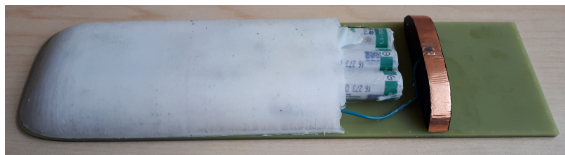
Figure 4.13: Partially potted SNs after curing the rubber.
