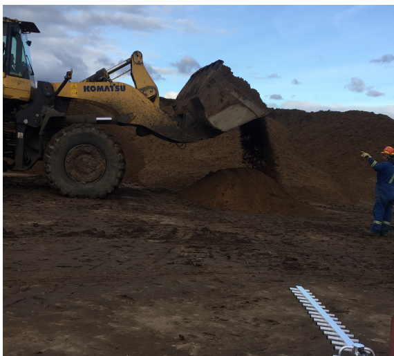
Figure 4.20: The SNs is on the ground underneath the sand being poured. Receiving antenna is 25 m away in the lower right corner
