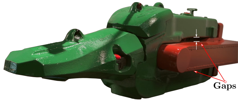
Figure 3.15: The shovel adapter and the gap exploited for wireless communication.
