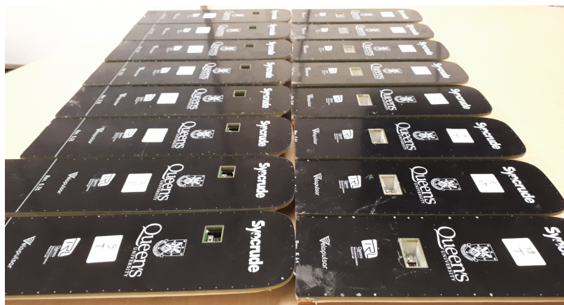
Figure 4.14: A batch of SNs before being covered with the fibreglass sleeve.
