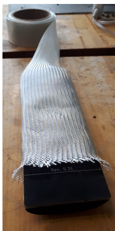
Figure 4.15: An SN being covered with the fibreglass sleeve.
