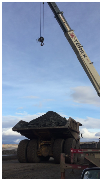
Figure 4.21: The SN is buried inside the truck's load. The sink and its antenna are hanging from an overhead crane on top of the hauler truck.
