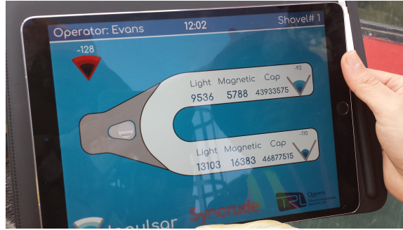
Figure 4.26: Operator dashboard on the cabin tablet. Sensor readings from both nodes are shown on their respective adapter’s arm along with their RSS in dBm on the right.
