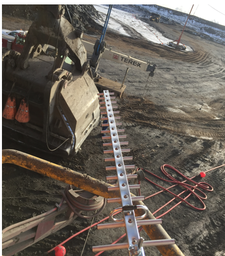
Figure 4.24: A photo from the sink node's location on a rail next to the cabin. The LoRa™ transceiver used a Yagi array for its high gain and directivity which added an extra 14 dB to the wireless link budget.
