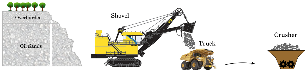
Figure 3.1: The first stage in an open-pit oil sands mining process.
