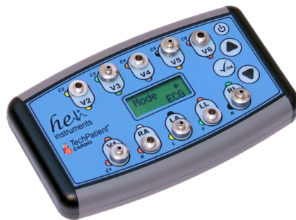
Figure 3.2: TechPatient CARDIO V4 ECG simulator
