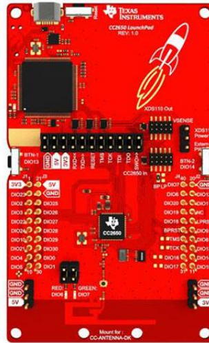
Figure 3.3: CC2650 SimpleLink multistandard wireless MCU
