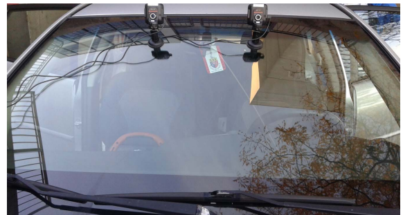
Figure 2. Cameras attached to the land vehicle (Hatchback) windshield for second trajectory recording.
