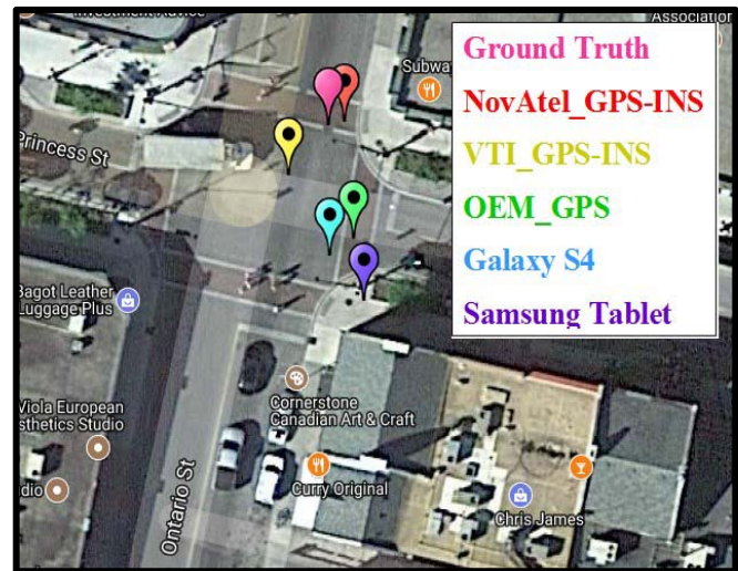
Fig. 16. 2-D road anomaly geo-referencing utilizing smart devices GPS receivers, OEM GPS receiver, integrated positioning solutions of VTI unit, and NovAtel SPAN unit, downtown area.
