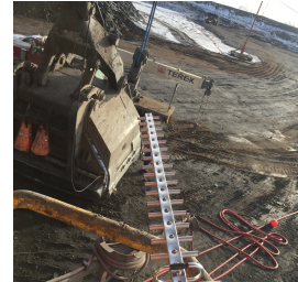
Fig. 8. A photo from the SiN's location on a rail next to the cabin. The LoRa™ transceiver used a Yagi array for its high gain and directivity which added an extra 14 dB to the wireless link budget.
