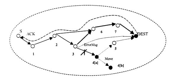
Figure 3.3 Destination/intermediate node has alternate path not passing through error initiating node
