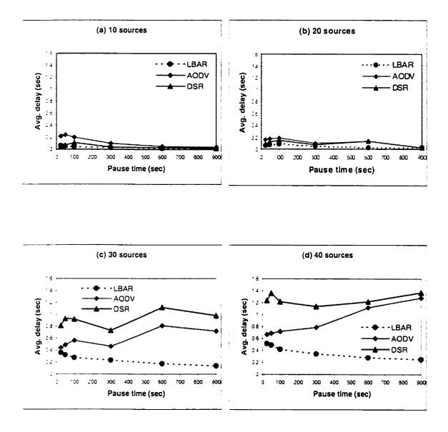
Figure 4.2: Average end-to-end delay for the 50-node model
