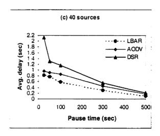
Figure 4.5: Average end-to-end delay for the 100-node model
