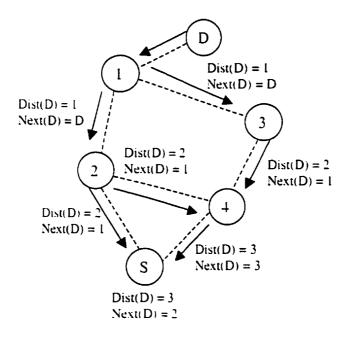
Figure 2.1 An example of Distance Vector Routing
