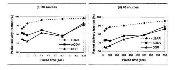
Figure 4.1: Packet delivery fraction for the 50-node model
