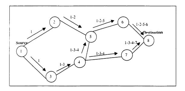
Figure 2.4 Building route records during route discovery in DSR
