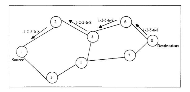
Figure 2.5 Forward back the reply message with route record in DSR
