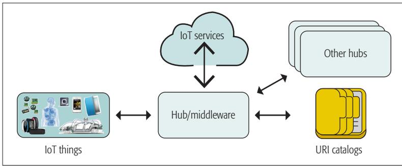
FIGURE 1. A hub architecture for Internet-based IoT (e.g., as adopted in Hypercat [4]).
