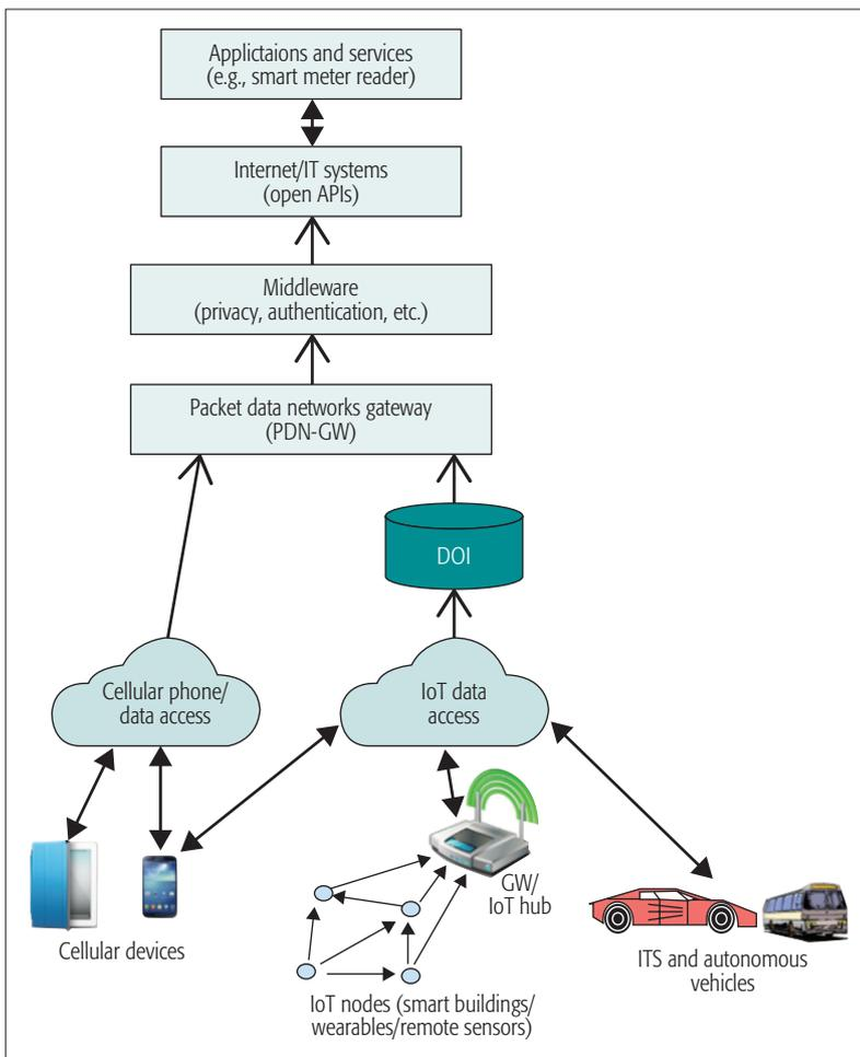
FIGURE 4. Proposed cellular-network-based IoT architecture with DOI module.
