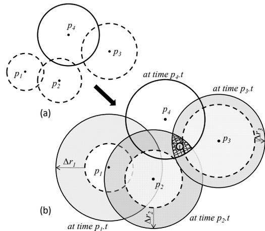
Fig. 3: Example on TSM technique. (a) The set of detections  $P = \{p_1, p_2, p_3, p_4\}$  for a tag  $t$  at different times within the same tolerance interval where  $p_4$  is the most recent. (b) The set of shifted detections after expanding  $p_1, p_2, p_3$  by  $\Delta r_1, \Delta r_2$  and  $\Delta r_3$  respectively, the tag  $t$  is expected to be in the shaded area.
