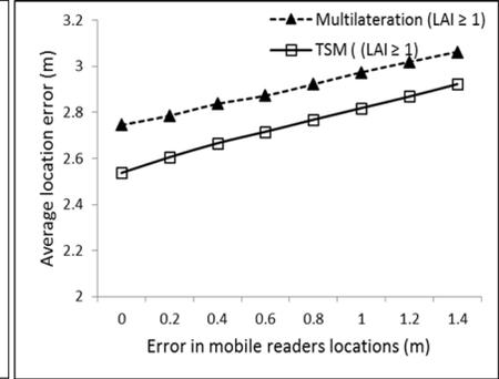
Fig. 8: Effect of error in readers positions on average location error (200 mobile reader).
