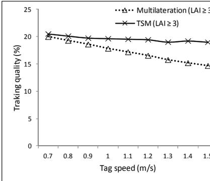
Fig. 10: Effect of tags' speed on tracking quality (200 mobile reader, 10s pause)
