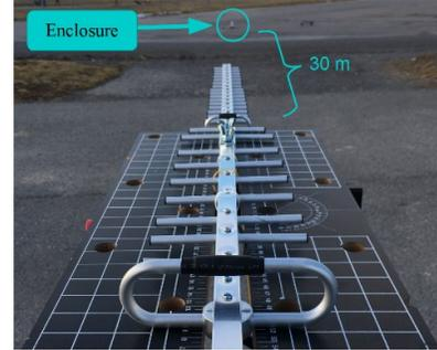
Fig. 7 The experimental setup showing the Yagi antenna at the receiver side and the enclosure 30 m away.
