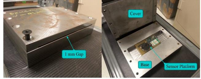
Fig. 5 The NHM enclosure model and the sensor platform inside its cavity.
