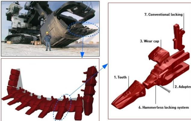
Fig. 2 An electric rope shovel (upper left), a set of adapters/teeth (lower left), and an adapter/tooth assembly (right) [16].
