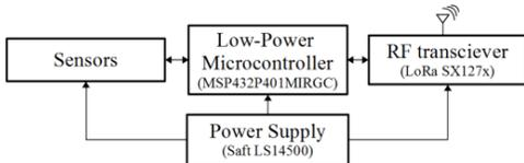
Fig. 3. Block diagram of the hardware sensor platform.
