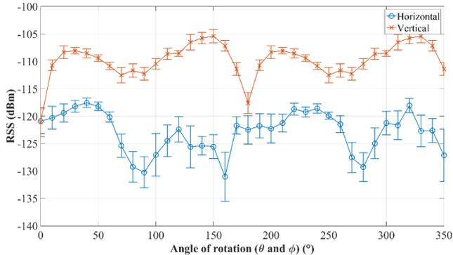
Fig. 9 Received signal strength at 30 m range for all angles around the enclosure when placed horizontally and vertically.
