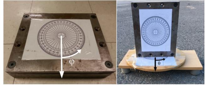
Fig. 8 The orientation of the enclosure with respect to the angle of rotation in the horizontal and the vertical position.
