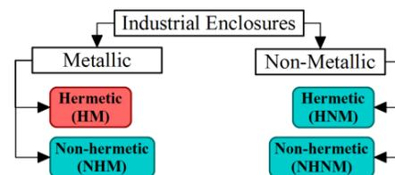
Fig. 1. Classification of industrial enclosures according to their material and type of concealment. The green types are the ones addressed by this work while the red is not.
