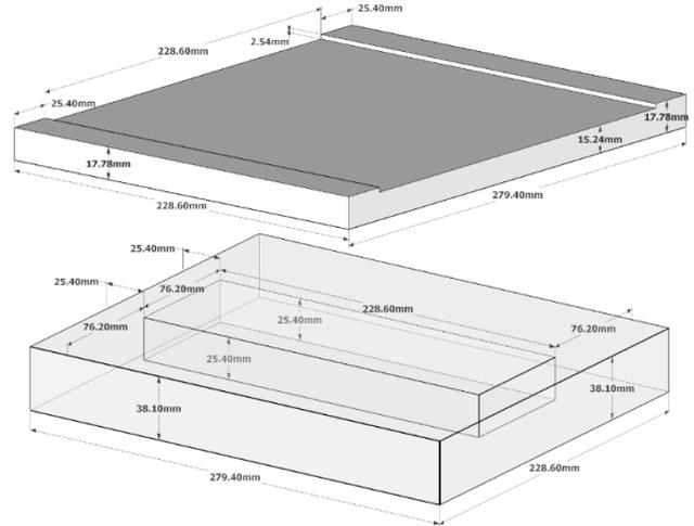
Fig. 6 CAD drawing of the enclosure model.
