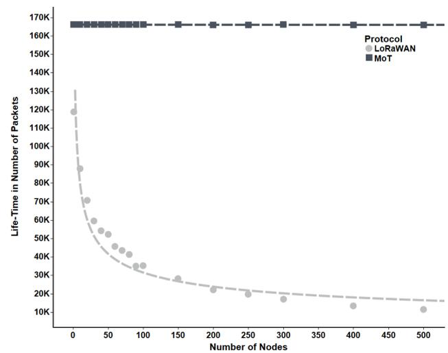
Fig. 4. Lifetime in packets of a single node using a 1 Ah battery, transmitting a single packet every 60 minutes, while varying the number of nodes in the network.
