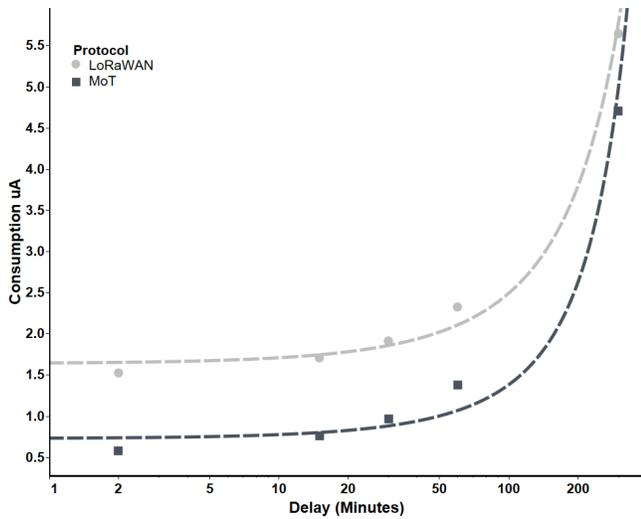
Fig. 2. Current consumption of successfully transmitting a single 1-Byte packet, with a single node in the network. (We used these results as a benchmark).
