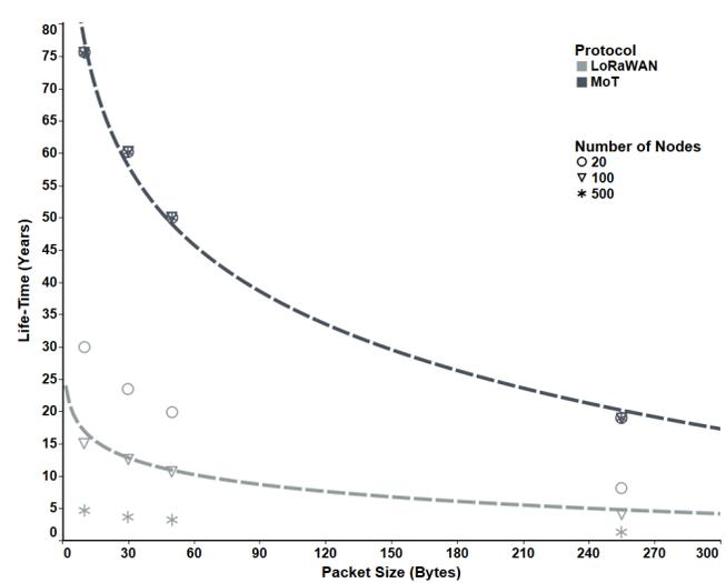
Fig. 5. Lifetime in years of a single node, transmitting one packet at different intervals while varying the number of nodes in the network.
