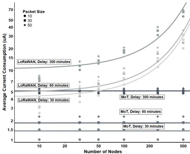
Fig. 3. Average current consumption of successfully transmitting a single packet, varying the payload size and number of nodes in the network.
