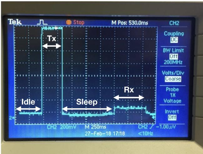
Fig. 1. Measured MoT Frame (Time values were modified for illustration purposes).
