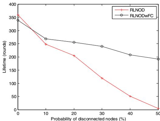
Figure 10. The average network lifetime in rounds vs. the probability of disconnected nodes in the monitored environment.
