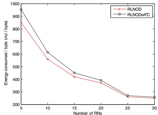
Figure 7. The average energy consumed per byte vs. the number of relay nodes.
