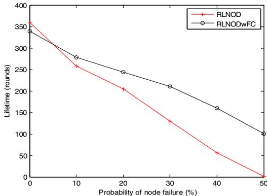
Figure 9. The average network lifetime in rounds vs. the probability of node failure in the monitored environment.
