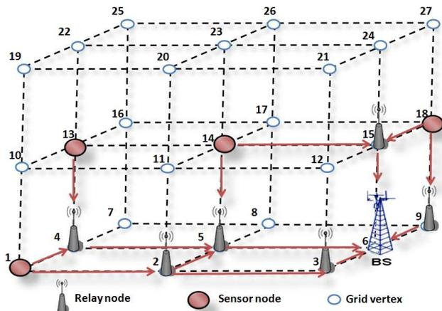
Figure 1. Sensors and relays are placed on the grid vertices to monitor specific event centers surrounded by the grid vertices in 3-D space.
