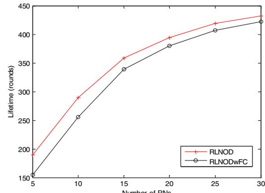
Figure 5. The average network lifetime in rounds vs. the number of relay nodes.
