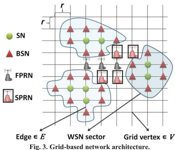
Fig. 3. Grid-based network architecture.
