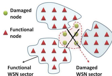
Fig. 1. Vast damage partitioning a WSN into disjointed sectors.
