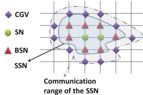
**Fig. 4. Communication range of a SSN, where CGV is a Covered Grid Vertex.**
