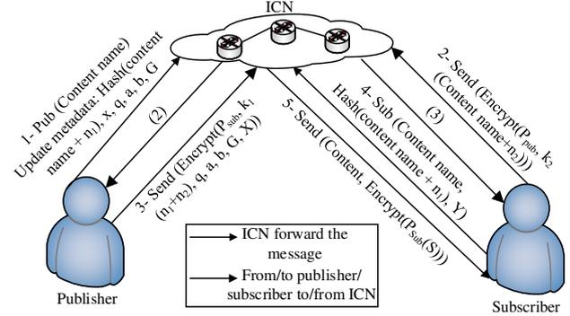
**FIGURE 2** Proposed decentralized access control protocol in ICN (ECAC)
