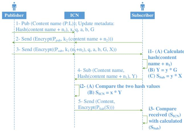
FIGURE 3 Sequence diagram of ECAC
