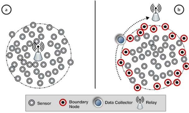
Fig. 2. A network model with (a) stationary relay and (b) with a mobile data collector.
