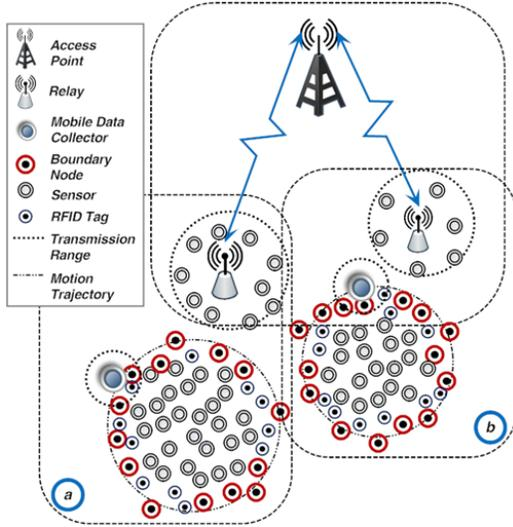
Fig. 1. A two-tier network architecture for RSN in public sensing.
