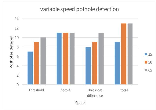
**Figure 4 – Pothole Detection Variable Speed**
