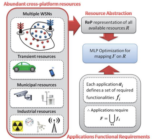
Figure 2. Optimal mapping of multiple applications over IoT resources across different platforms
