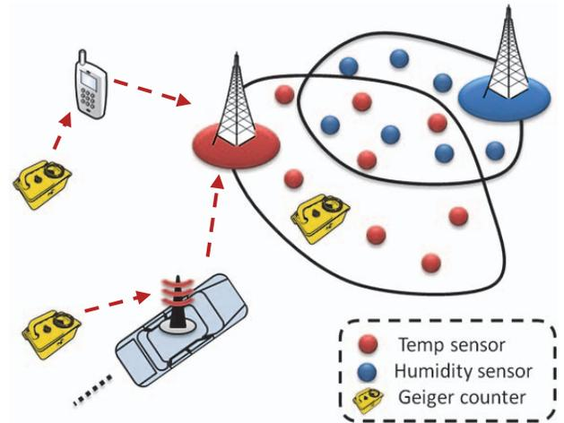
Figure 3. Use case for resource utilization in IoT involving a WSN for temp monitoring (in red), Humidity monitoring (in blue), Geiger counters present in a large region, and two common transient resources (vehicle and smartphone)
