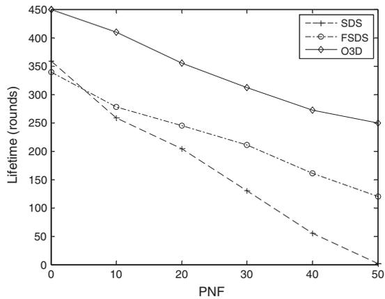
Fig. 2. Lifetime as a function of Probability of Node Failure (PNF).
