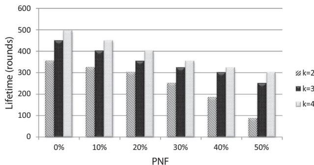
Fig. 8. Lifetime vs. the probability of node failure under three different fault-tolerance levels;  $k = 2, 3,$  and  $4$ .
