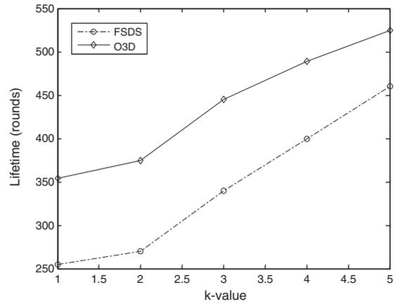
Fig. 4. Lifetime as a function of fault-tolerance level  $k$ .
