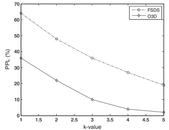
Fig. 5. Packet loss as a function of the fault-tolerance level  $k$ .
