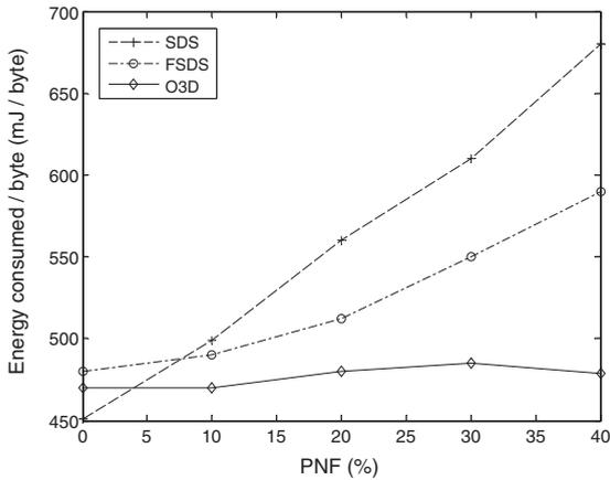
Fig. 6. Energy consumed vs. the Probability of Node Failures.
