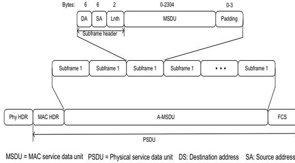
Fig. 2. A-MSDU aggregation frame structure
