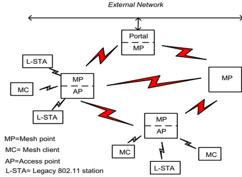
Fig. 1. Wireless mesh network's components and hierarchy structure
