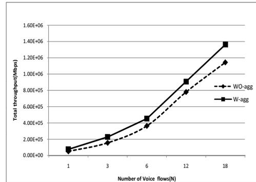
Fig. 12. The achieved throughput for increasingly voice network traffic load
