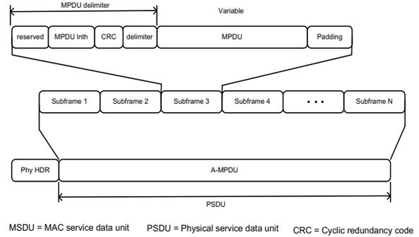
Fig. 3. A-MPDU aggregation frame structure
