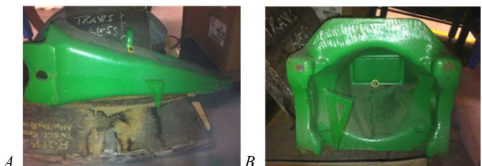
Figure 2. A. Ground Engaging Tool (GET), or shovel tooth B. Location of Sprouts sensor platform inside the GET
