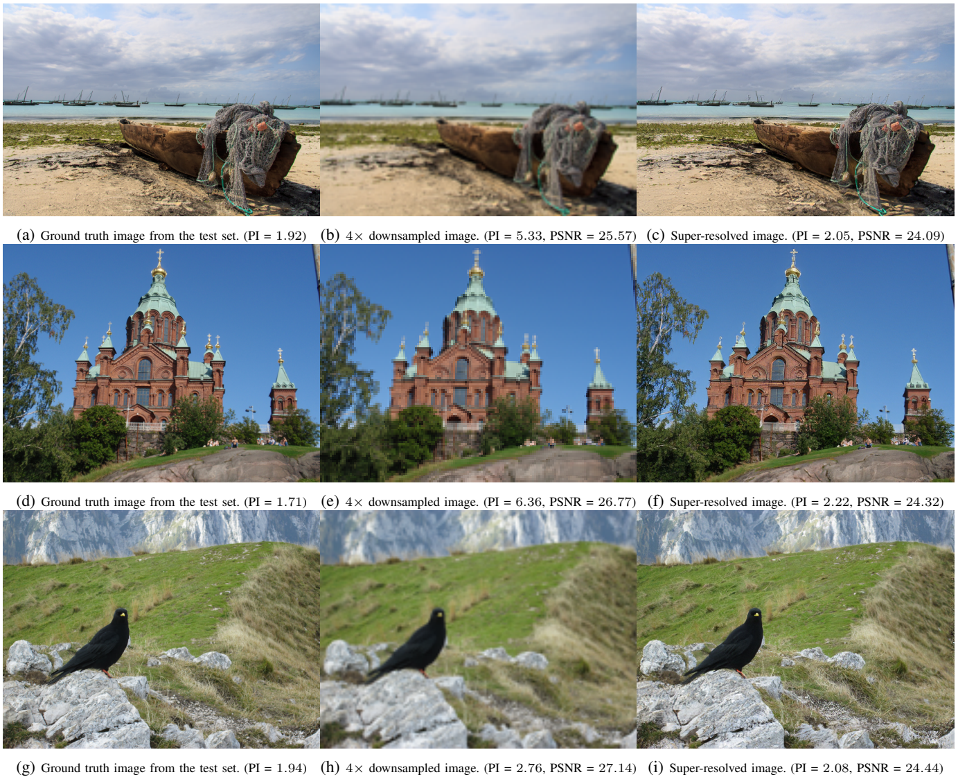
Figure 2: Qualitative results of SR tasks of three different images from the PRIM dataset [12]. The resulting images can be evaluated visually by comparing it with the ground truth image. The PI and PSNR scores, used in PIRM-SR challenge [12], are used to assess the quality of the super-resolved images. The results show more natural textures, e.g., bird’s feather, building structure and grass texture.
