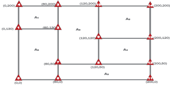
Fig. 6 Warehouse model with six non-uniform sensing areas with 14 numbered anchor nodes placed in the corners
